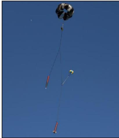
For the payload ballast, 1.93lbs was used through flight and recovery. In addition to the ballast, the payload bay contained the spring ejection systems that will be used in the competition launch. Assembling the rocket before the launch as well as the test launch itself demonstrated that the spring ejection systems were fully compressed within the airframe. This indicated that oscillations in the springs would be non-existent, and therefore are not a concern for flight.
